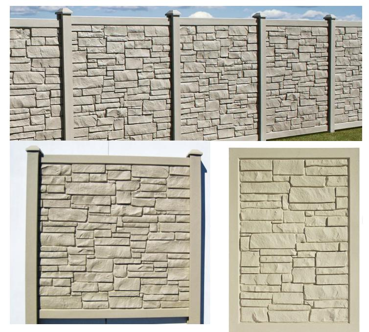
Proposed fencing made of 'BuffTech Allegheny Beige Granite' is made of recycled polyethylene and is reinforced with steel. This fencing is the standard for K9 across the country as it is nonporous, unlike masonry, so it can be disinfected and cleaned to eliminate odor and bacteria; dampens sound better than masonry; and is 8' tall to further buffer sound rather than the standard 6' fencing.
