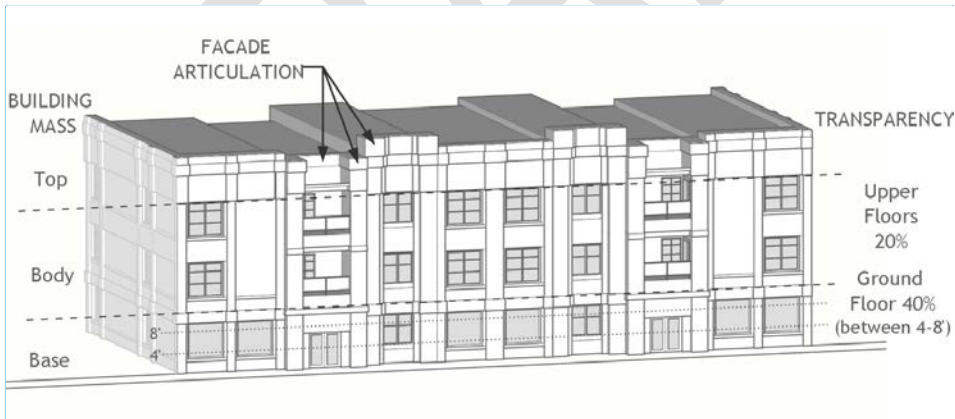
Figure 2-121.GF: Façade Articulation, Building Form, and Transparency
